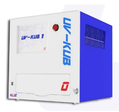
Kloé has extensive experience in photolithography through its Dilase direct laser writing technology, and thus introduces the UV-KUB system for the curing of UV light photosensitive materials. The UV-KUB is a simple exposure system based on UV LED with available light sources at 365 nm or at 405 nm, depending the version. This is a very compact table-top system capable of exposing up to 4 inches diameter wafer
