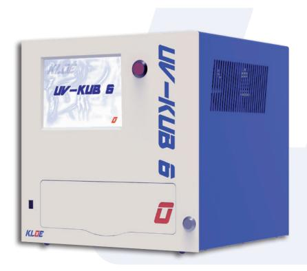
After the worldwide success of the UV-KUB 2, Kloé introduces the extended version capable of exposing up to 6 inches diameter wafer. The UV-KUB 6 is an exposure and masking system based on UV LED with available light source at 365 nm for the curing of UV light photosensitive materials. This is a very compact table-top system compatible with hard (physical) or soft (proximity) contact processes, and features variable mask to substrate distance control.
