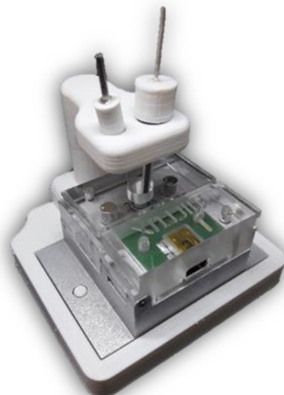
Platform with external reference & auxiliary electrodes
